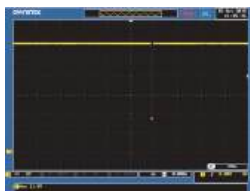
SEQ6: Momentary Drop in Supply Voltage
